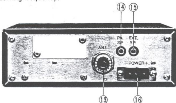
13. **ANTENNA CONNECTOR** — This female connector permits connection of the transmission line cable male connector (PL-259) to the transceiver.
