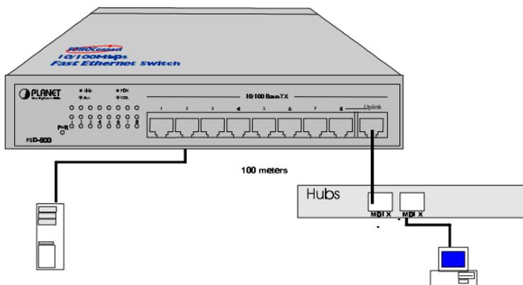
Figure 3. 100Mbps File server to Hubs Connection
