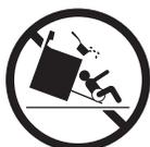
**To reduce the risk of tipping, the appliance must be secured by properly installed anti-tip bracket provided with the unit. Refer to the Installation Instructions for proper anti-tip bracket installation.**
