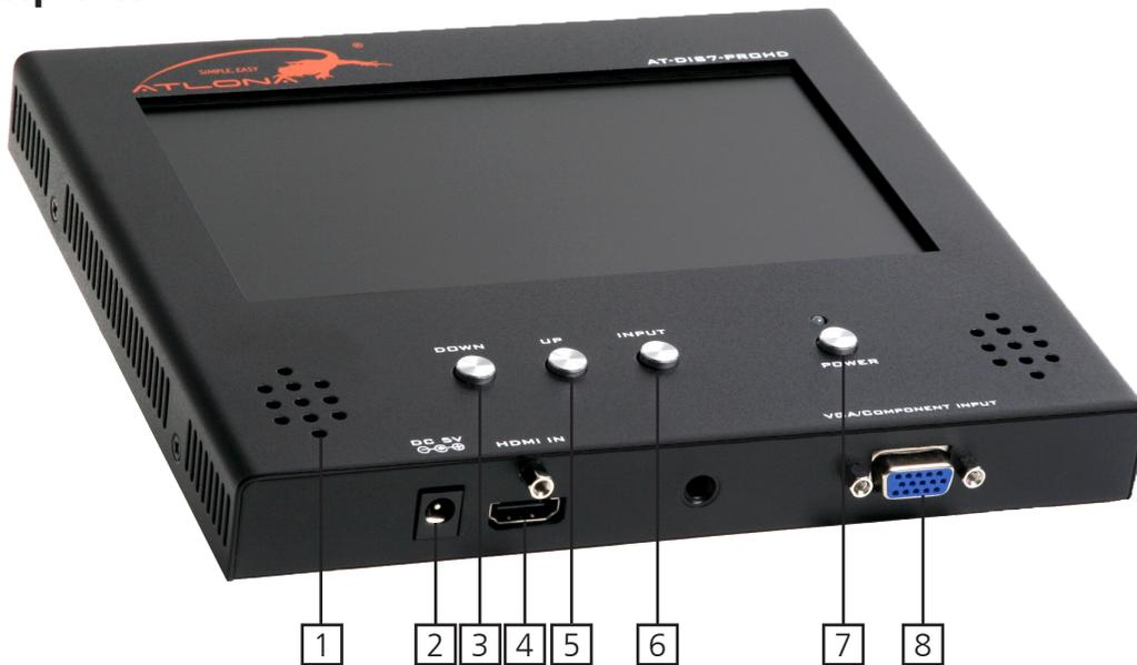
1. Output Speakers: These are the two built-in 2Channel speakers.
