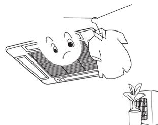
Be sure to install the air filter, ensure that the air filter is not dirty. Otherwise may result in machine damages or cause malfunction due to dust inside the unit
