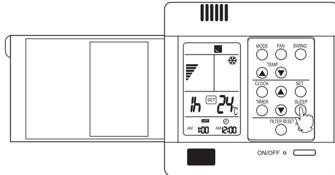
Press SLEEP button once to make the air conditioner have the previous-set sleep time (first power-on is "1h"), the sleep symbol will appear. Press time button ▲/▼, you can choose the time in 1~8 hours. Each press of▲/▼, the time increases/reduces 1 hour and "xh" appears in the humidity setting part, "OFF" appears in "TIMER OFF" display part and timer-off time; press SLEEP button again to cancel sleep function, the sleep symbol disappears.
