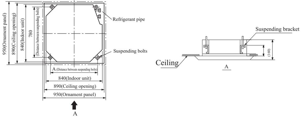
(2) Cut an opening in ceiling for installation if necessary. (when ceiling already exists.)
