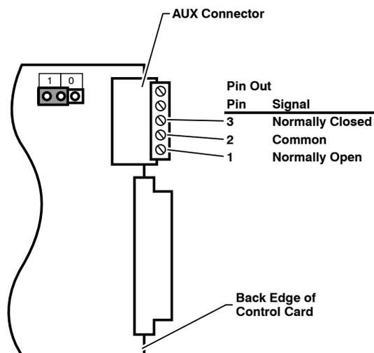
**Figure 7.1: Control Module AUX Connector - Output Contacts**
