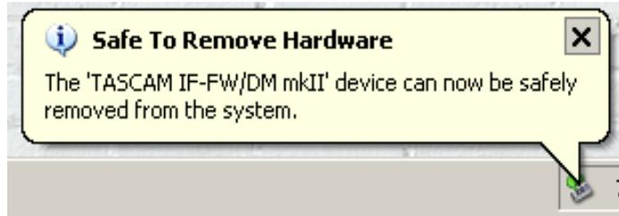
After using the “Safely Remove Hardware” function of Windows to stop the IF-FW/DM MKII, you will see “1394: Driver Offline” reported in the mixer’s DIGITAL status screen for the IF-FW/DM MKII.
