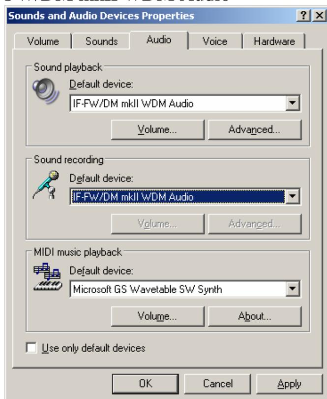
Note that audio supplied through WDM and routed to the IF-FW/DM MKII in this way will be summed to any audio being supplied via ASIO, so always check that Windows Sounds will not interfere with your regular DAW recording or mixing sessions. For a computer dedicated to audio, TASCAM recommends turning off all Windows sounds. Navigate to Start→Control
