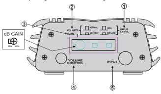
The switches and gain settings are located behind a watertight pulg, which also lights up when the amplifier is on. Be sure to replace the plug when finished with adjustments
