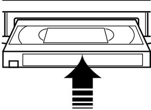
The VCR automatically turns on. If the erase-protection tab has been removed from the cassette, playback automatically begins.
