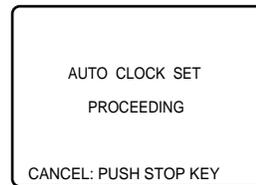
It takes up to 10 minutes for the VCR to set the clock using the EDS signal. If the VCR finds a signal, it automatically sets its clock to the correct time, and **AUTO CLOCK SET COMPLETED** appears. If the VCR does not detect a signal within this time, **AUTO CLOCK SET INCOMPLETE** appears. There is probably not an EDS signal available in your area. Press **MENU**, then see "Manually Setting the Clock" on Page 16 to set the clock.
