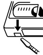
If you want to record on a video cassette that does not have the tab, put a piece of heavy plastic tape over the erase-protection tab hole.
