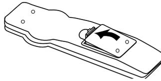
**Note:** When the remote control stops working or operates poorly, replace both batteries.
