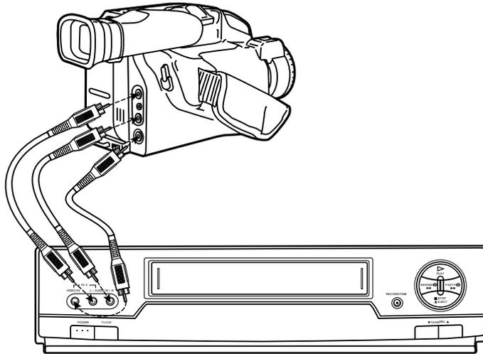
1. Insert the plugs at one end of the cable into the **AV 2 L-AUDIO IN-R** and **AV VIDEO IN** jacks on the Model 63's front panel, or the **AUDIO IN/VIDEO IN** jacks on the Model 114's front panel.
