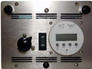
Figure 1: Ventilation Timer & Humidity Control
