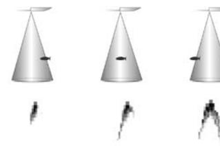
Transducer Cone and Fish Arches
