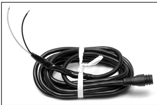
**Strip the ends of the VHF radio's data wires. Connect them to the pre-stripped wires of the M68i's data cable (shown right).**
