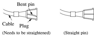
Before plugging the UHF/VHF Rod Antenna (Supplied with 13" model only) into the ANT(enna). IN jack, check that the pin is not bent. If it is bent, straighten the pin as illustrated, then plug the pin into the ANT(enna). IN jack.
