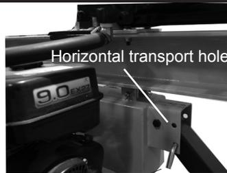
Close-up of Push Pin (26) securing the Front Leg Assembly (11) to the bracket on the Oil Tank Assembly (10B).
