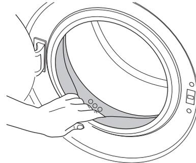
If the holes on the bellow shown in the figure is blocked, open the holes using a toothpick.
