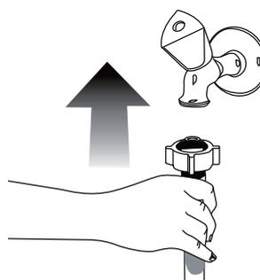
3. Open the taps completely after making the hose connection to check for water leaks at the connection points. If any leaks occur, turn off the tap and remove the nut. Retighten the nut carefully after checking the seal. To prevent water leakages and damages caused by them, keep the taps closed when the machine is not in use.
