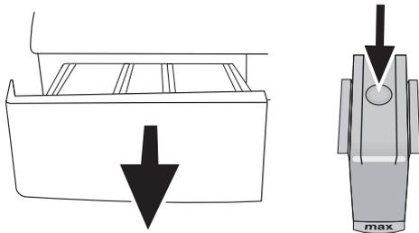
1. Press the dotted point on the siphon in the softener compartment and pull towards you until the compartment is removed from the machine.
