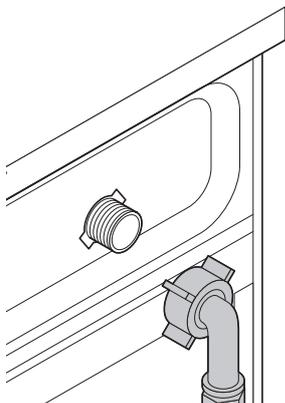
2. Tighten all hose nuts by hand. Never use a wrench when tightening the nuts.
