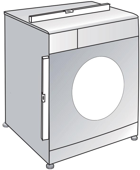
1. Loosen the lock nuts on the feet by hand.
