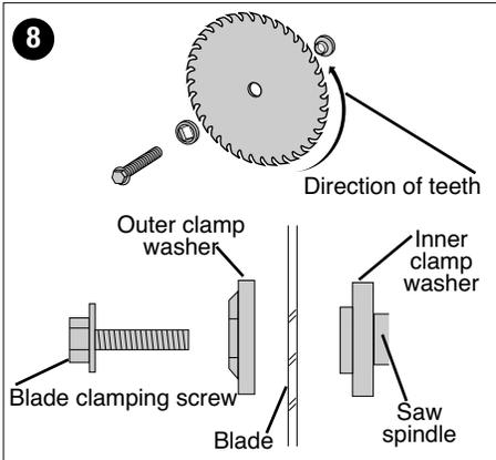
Tighten blade securely as shown (**figure 9**). Use scrap wood to prevent spindle rotation.
