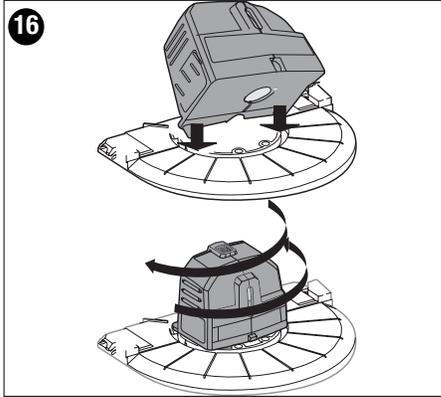
**(2) Fixed Position** - To use the laser in the fixed position, place the rear legs in the holes on the protractor. Refer to figure 17 for the angles created when using the laser in these holes.
