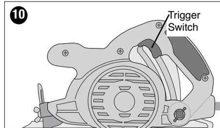
To turn the tool off, release the trigger switch. There is no provision for locking the tool on, and the switch should never be locked on by any other means.
