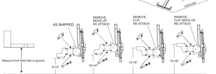
ORIENTATION OF CLASS 2 and CLASS 3 HITCH ADAPTERS IS IDENTICAL
