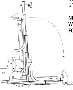
TO ERECT THE TILT AND TOTE BACK TO ITS TRAVEL POSITION, SIMPLY ROTATE UPRIGHT, AND REPLACE THE HITCH PIN.
