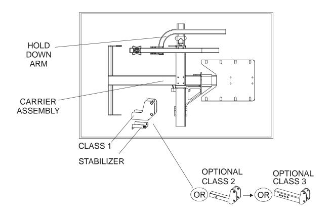
Each Tilt and Tote is packaged with a Class 1 Hitch Adapter and Stabilizer. If a Class 2 or Class 3 hitch adapter is required, separate parts must be ordered.
