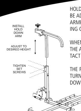
HOLD DOWN ARM HEIGHT CAN BE ADJUSTED SO THAT WHEELCHAIR'S ARMRESTS CLEAR ARM WHEN LOAD-ING ONTO A TILTED PLATFORM.
