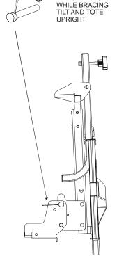
ONCE PIN IS REMOVED, THE TILT AND TOTE CAN BE LOWERED JUST BELOW PARALELL WITH THE GROUND BEFORE RESTING ON ITS MECHANICAL STOPS.
