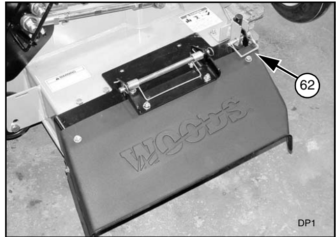
Figure 4. Discharge Chute with Adapter Installed
