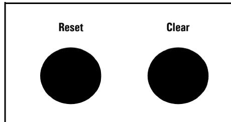
3. Release the Reset button and wait for about one second for the Self-Test LED to start flashing.
