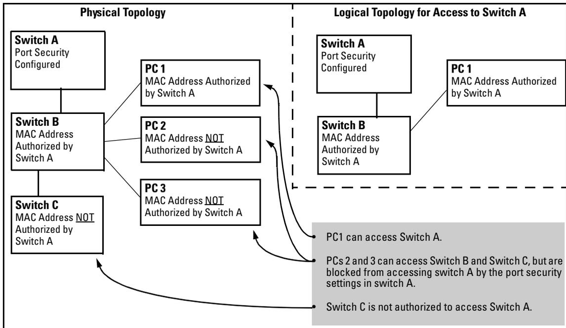
Figure 9-1. Example of How Port Security Controls Access
