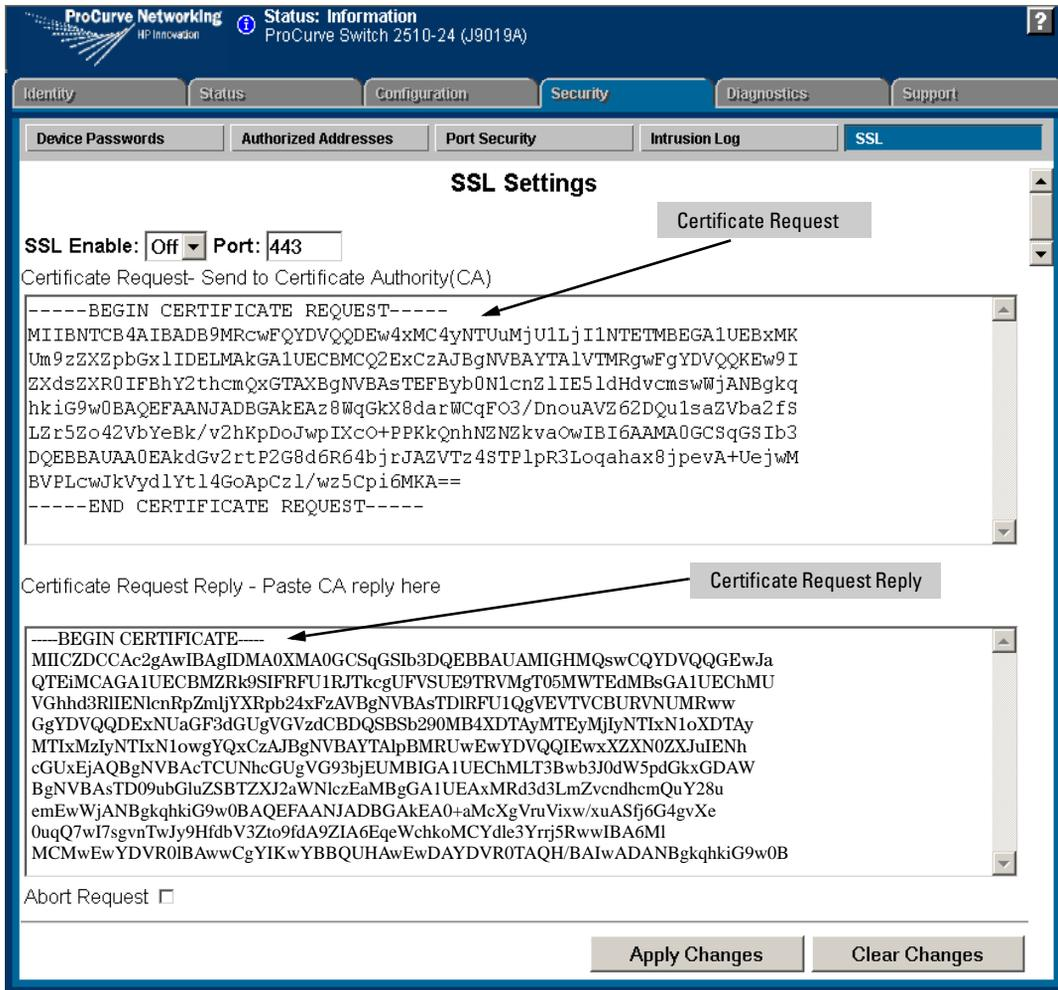
Figure 7-7. Example of a Certificate Request and Reply
