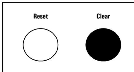
Figure 2-5. Press the Clear Button for One Second To Reset the Password(s)
