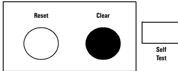
4. When the Self-Test LED begins flashing, release the Clear button
