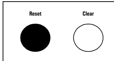
2. While holding the Reset button, press and hold the Clear button.
