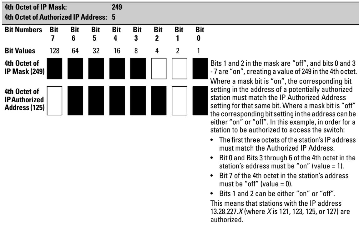
**Figure 10-5. Example of How the Bitmap in the IP Mask Defines Authorized Manager Addresses**
