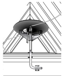
**Note:** Even with the advanced design of this antenna, large obstructions such as canyon walls, mountain sides, and other man-made or natural geographic objects can impair performance. Therefore, it is best to minimize any obstructions that block the "line of sight" by mounting the DBS antenna on the roof or on the highest possible point.
