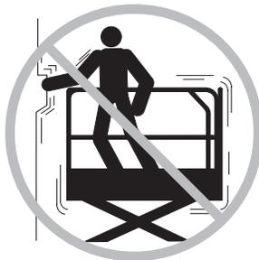
Do not modify or alter an aerial work platform without prior written permission from the manufacturer. Mounting attachments for holding tools or other materials onto the platform, toeboards or guard rail system can increase the weight in the platform and the surface area of the platform or the load.
