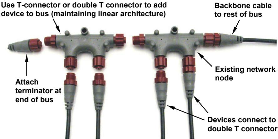
In this example, a new device is added to the NMEA 2000 bus by installing a T connector between a T connector and a terminator at the end of the backbone (network bus).
