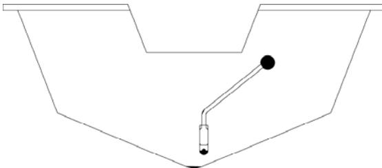
**Temp module on transom with cable routed through the transom. Notice that the sensor was routed so the smart module is inboard.**
