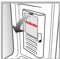
**ODOUR FILTER\***: Some models are fitted with a new odour filter with active carbons, which ensures better air quality inside the refrigerator.
