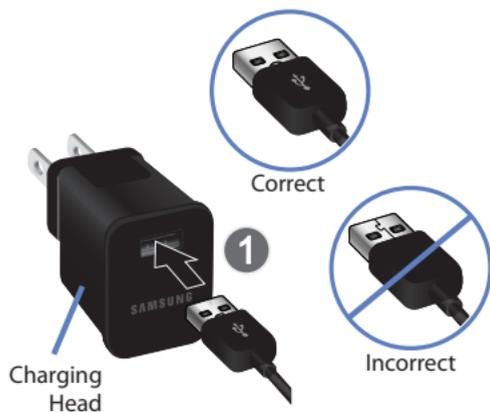
2. Insert the USB cable into the device's Charger/Accessory Port (2).
