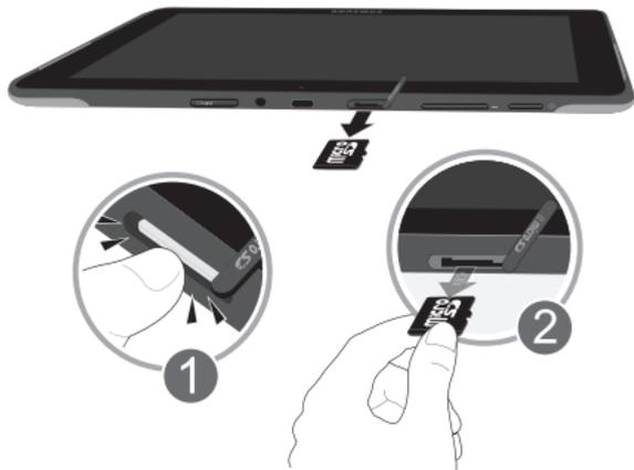
4. Gently press down on the memory card (1), so that it pops out from the slot, and carefully pull the card out (2).
