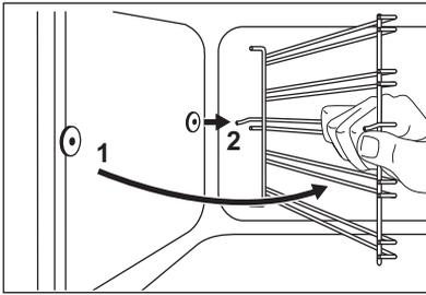
2. Pull the rear end of the shelf support away from the side wall and remove it.
