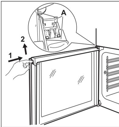
1. Push the door trim at one side to remove it. Refer to the diagram.
