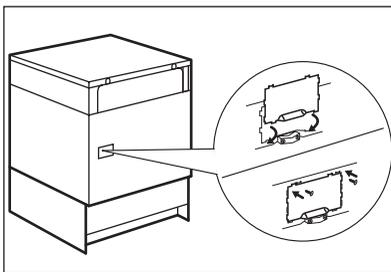
The recommended cross-section area is six square millimetres (6 mm<sup>2</sup>). When you refit the mains terminal cover, make sure that the lower tabs are located inside the bottom edge of the aperture, before you fix the two screws into the top edge of the mains terminal cover. Make sure that the cover is securely fastened.
