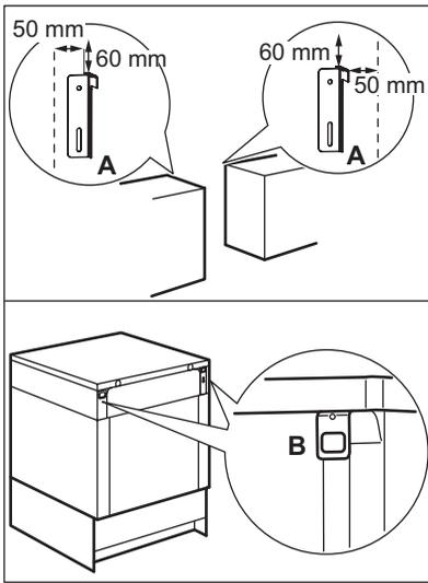
1. Set the correct height and area for the appliance before you attach the anti-tilt protection.
