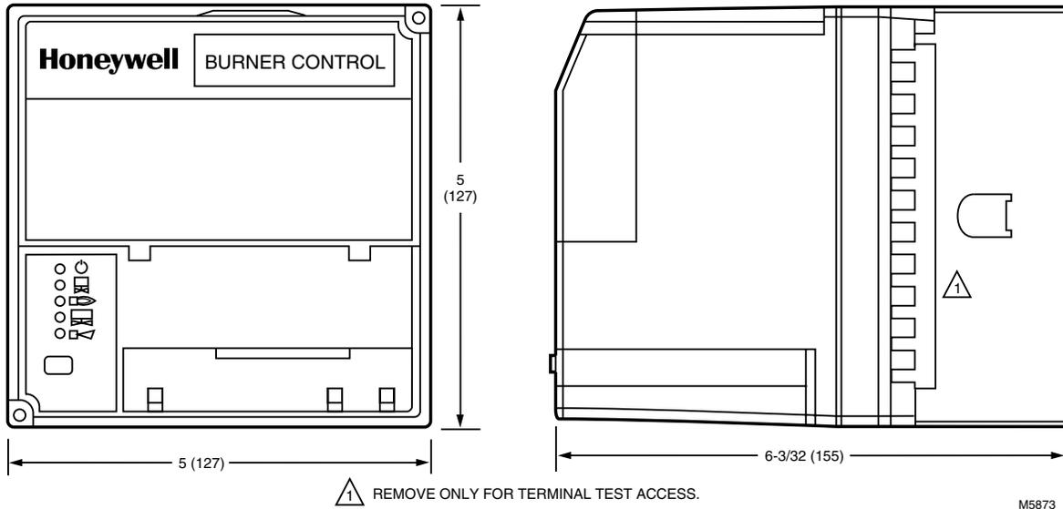
**Fig. 2. Mounting dimensions of RM7824A Relay Module and Q7800B Subbase in in. (mm).
