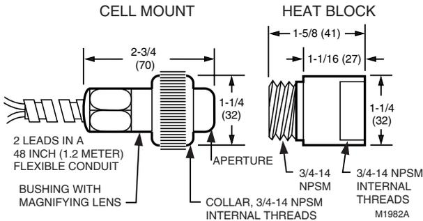
**Fig. 3. Infrared detector dimensions in in. (mm).**
