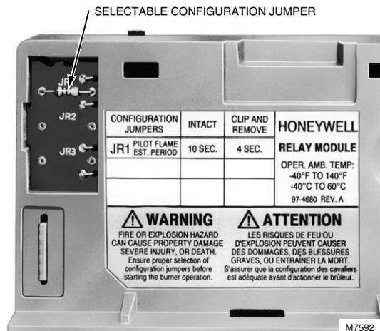
Fig. 15. Selectable site-configurable jumpers.
