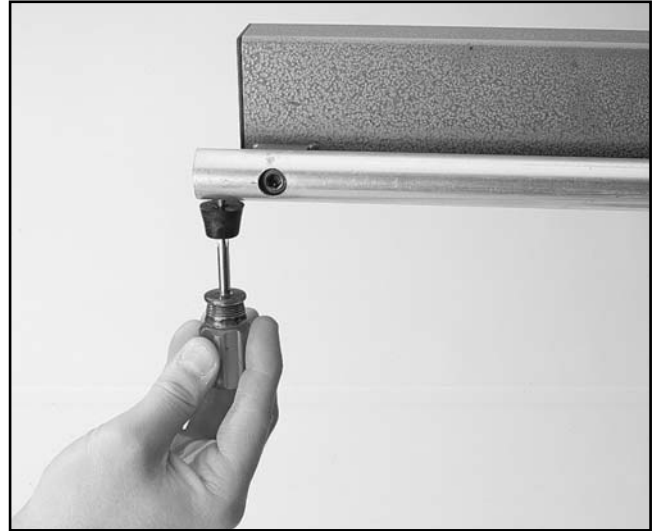
Figure 10. Rear stop installation.
