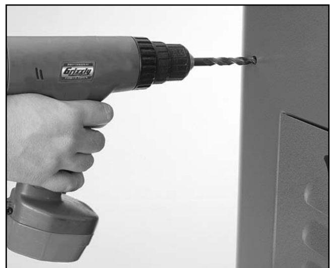
Figure 3. Drilling the mounting holes.
