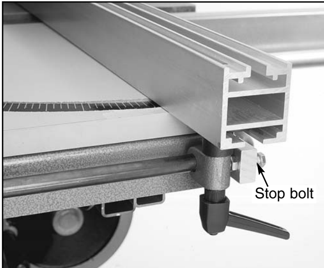
Figure 16. Adjusting positive stop.
