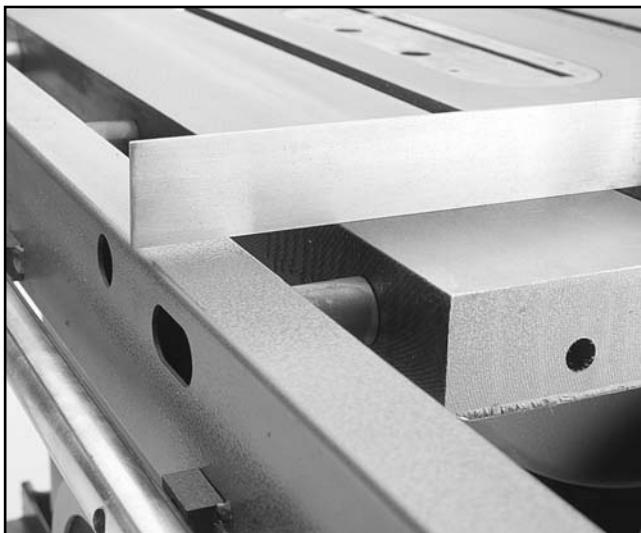
Figure 2. Aligning the upper rail.
