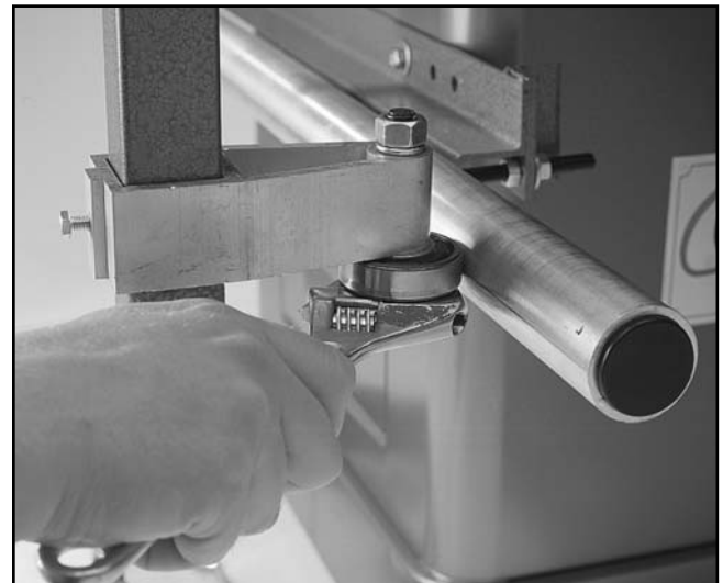
Figure 15. Adjusting the lower guide.
