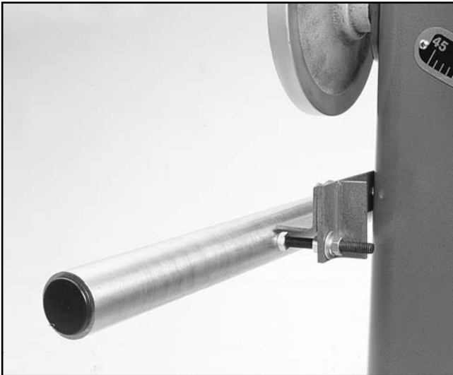
Figure 5. Mounting the lower rail.
