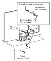
The length of the M6 eye bolt differs depending on the rope or chain diameter. Please see below illustration.
