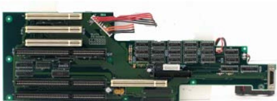
Take care not to uncouple any cable connectors while installing accessory boards, and be sure the boards you are installing are fully seated into the appropriate connectors. Re-install the upper card edge bracket after installing new circuit boards.
