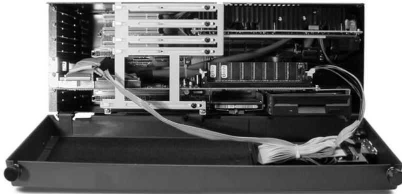
As you will notice in the photo below, we removed the backplane circuit board from the D4-470 case to facilitate viewing. *Do not* remove the backplane board to install expansion boards.
