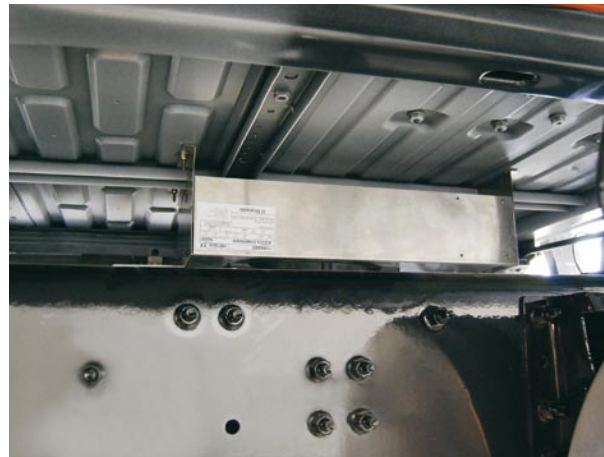
Figure 2a - Condensing unit mounted under truck
