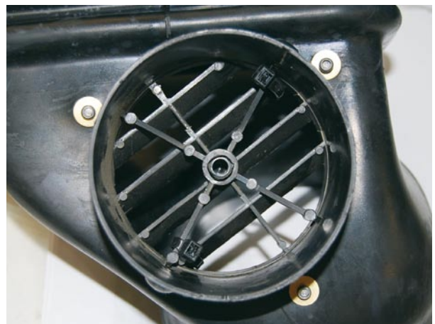
Figure 15b - V4 RND black installed in the duct transition
