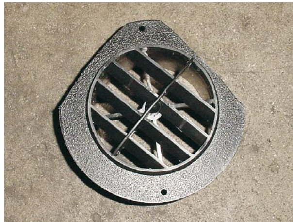
Figure 14 - V4 RND trimmed to fit
