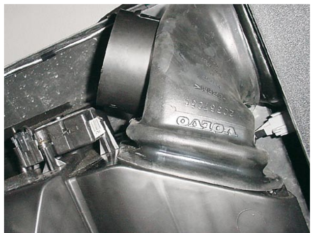
Figure 16 - Duct transition reinstalled
