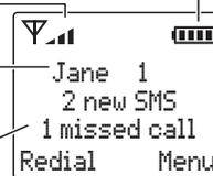
The battery charge level. When this shows 'nearly empty'
