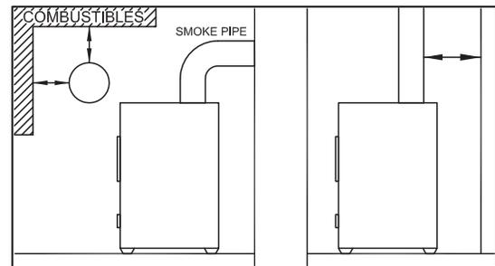
According to NFPA standards, single wall stove pipes can be within 9" of combustibles provided an approved fire retardant material covered with 28 gauge sheet metal, spaced out 1" on non-combustible spacers, is utilized. See illustration.
