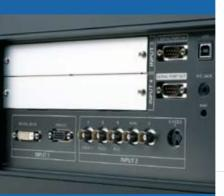
▲ The LW600 offers input flexibility by providing two option board slots to allow for additional signal connectivity from a variety of option cards.
