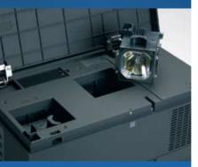
▲ The LW600 new dual lamp design provides high brightness and increased uniformity even in a single lamp mode.
