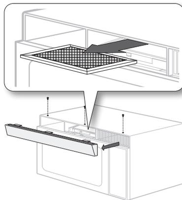
6. Slide a new charcoal filter into place. The filter should rest at the angle shown.
