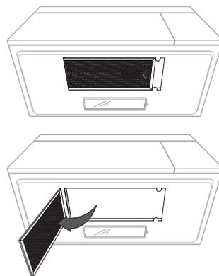
2. Soak the grease filter in hot water and a mild detergent. Rinse well and shake to dry.
