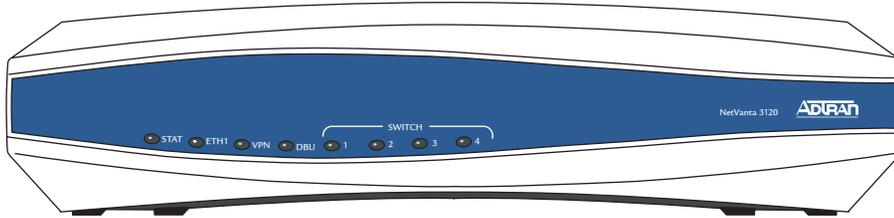
**NetVanta 3120 Front Panel Layout**
