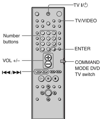
Press and hold TV I/II while entering your TV's manufacturer's code (see the table) using the number buttons and press ENTER. Then release TV I/II.
