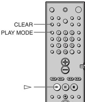
**1** In stop mode, press **PLAY MODE** repeatedly until “SHUFFLE” appears on the front panel display.
