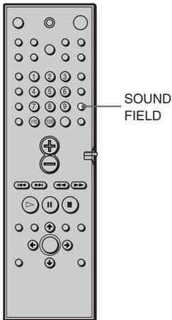
**Press SOUND FIELD  $-/+$  on the system or SOUND FIELD on the remote repeatedly until “AUTO DECO.(AUTO DECODING)” appears on the front panel display.**
