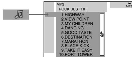
When the list of all tracks or albums cannot be displayed on the window, the jump bar appears. Press  $\rightarrow$  to select the jump bar icon, and then scroll the jump bar to display the rest of the list using  $\uparrow/\downarrow$ .
