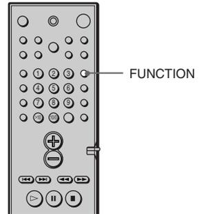
**Press FUNCTION repeatedly until VIDEO 1 or VIDEO 2 that you connected the unit to appears on the front panel display.**
