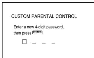
Enter a 4-digit password by using the number buttons, then press ENTER. The display for confirming the password appears.
