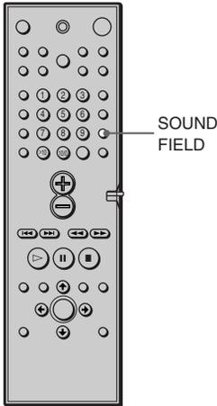
Press **SOUND FIELD +/-** on the system or **SOUND FIELD** on the remote repeatedly until “**2CH STEREO**” appears on the front panel display.
