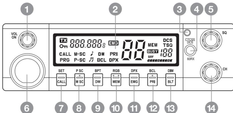
1. Rotary On / Off Switch and Volume Control
