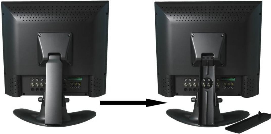
2. Connect the Power Cable, Cameras, Ethernet Cable and any Alarm Devices to the System by running the cables through the hole in the stand before connecting to the Observation System.
