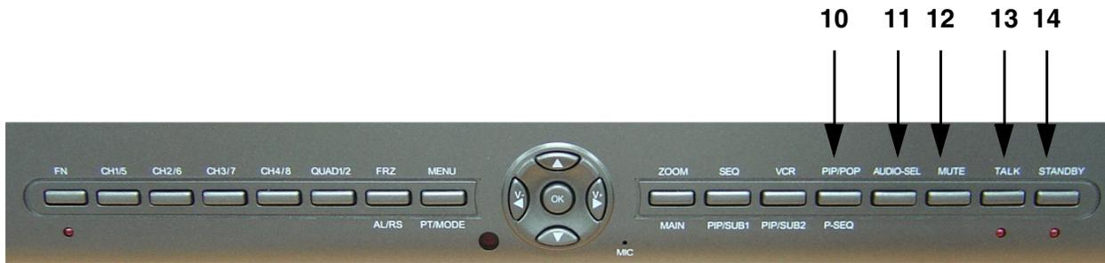
10. **PIP POP BUTTON** - Display a main camera image with secondary camera sub-images:
