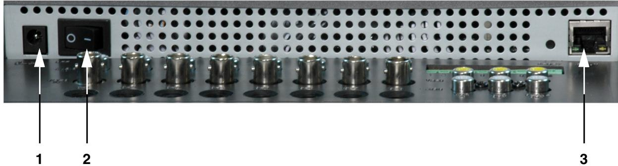
1. **AC INPUT** - Connect the AC power (using the power cord provided with the unit) from the monitor to an electrical outlet
