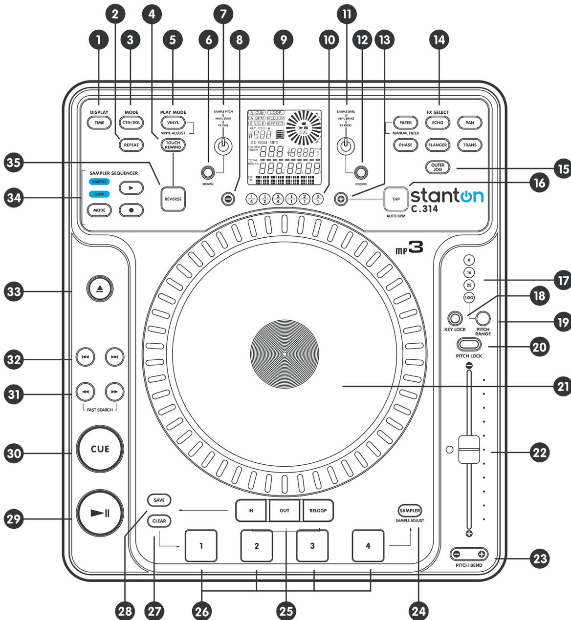
1. **TIME** – Switches the time value displayed in the LCD between elapsed track time, remaining track time, and the total remaining time for the entire disc. Markers next to the time readout indicate which of these modes is enabled.
