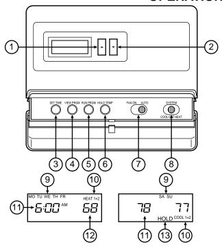
Figure 6. Thermostat display, buttons, and switches
