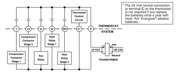
Figure 3. Typical wiring diagram for single transformer systems
