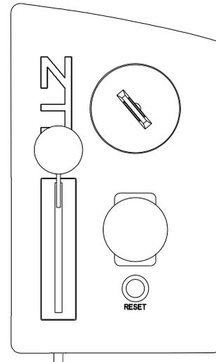
**NOTE:** While mowing, "blade(s) engaged", throttle control must be set to the **MAXIMUM** or wide open setting to insure adequate cooling of the engine and to maintain mower deck blade speed.
