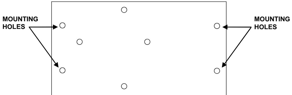
U-clamps or lag screws may be used for permanent mounting
