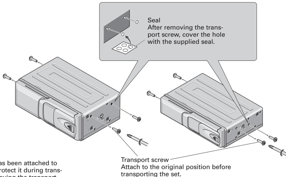
A transport screw has been attached to the set in order to protect it during transportation. After removing the transport screw, cover the hole with the supplied seal.
