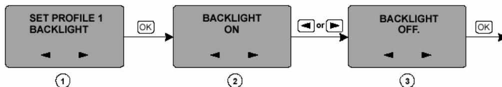
To switch the backlighting ON/OFF:
