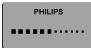
When the handset is in the charger, the charging progress is indicated by a flashing red LED on top of the handset. The charge status is also indicated in the display. Completion of the charge cycle is indicated by switching ON the red LED continuously and the display will return to normal mode.
