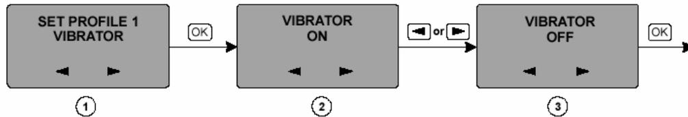
To switch the vibrator ON/OFF:
