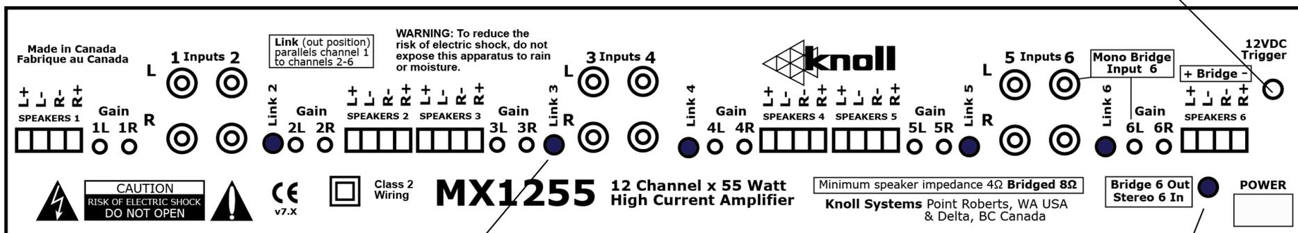
The Link button is normally set to the "in" position to give all six stereo inputs individual sources. When the Link button is set to the "out" position, that input Left/Right is linked or cascaded (or paralleled) to input #1 (without the use of Y cords). Any or all combination of linked inputs 2 to inputs 6 are possible. When all inputs are linked to input 1 the input impedance is about 4000 Ω.
