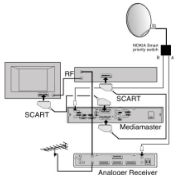
Both the VCR and the analogue satellite receiver must be tuned to different UHF channels (than the Mediamaster) when using RF-connectors.
