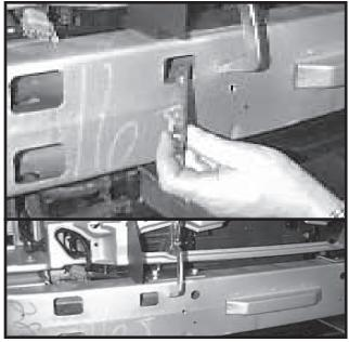
9. Slide nut plate thru bumper hole and fasten with 3/8" x 1-1/4" bolts, and lockwashers.
