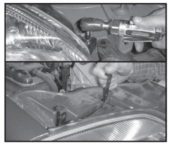
3. Remove headlights, one bolt in front and two L-shaped fasteners in back, pull these staight up. Pull headlight out and unplug wiring.
