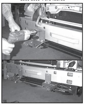
10. Fasten angle bracket, with 3/8" x 1-1/4" bolts, flatwashers, and lockwashers to pod and loosely tighten. Drill 5/16" hole in center of bumper using angle bracket as template. Attach here with 3/8" self threading bolt. Tighten all previously installed bolts for pods at this time.
