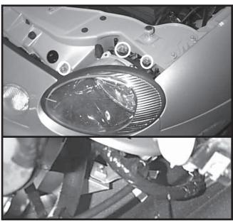
3. Remove lower headlight pod bolt (from each side), located approximately 6 inches above horn bracket. Remove three top headlight bolts and loosen long headlite bolt. Unplug and remove headlite.
