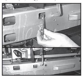
9. Slide nut plate thru bumper hole and fasten with 3/8" x 1-1/4" bolts, and lockwashers.
