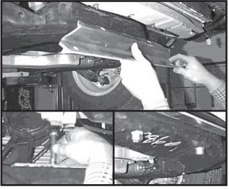
11. Attach subframe mount ('99 model uses narrow mount) with 1/2" x 4" bolts, lockwashers, and nuts on bottom side.
