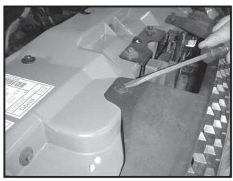
Remove grill, four plastic push fasteners, lift up and out. Remove two plastic push fasteners from top of facia and remove facia.
