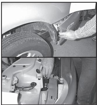
Pull front facia out on each side by wheelwell, and lift up on metal edge across the front. Pull forward and unplug turn signal lites, and side marker lites.
