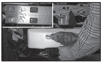
Remove front bumper styrofoam by drilling out pop-rivets, and set aside.
