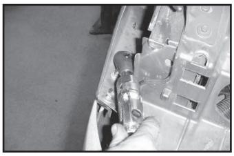
4. Remove two more bolts, fender to facia, by head-light openings.
