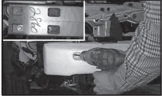
6. Remove front bumper styrofoam by drilling out pop-rivets, and set aside.
