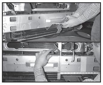
7. Slide each pull ear pod starting from center of bumber out and measure approximately 1-9/16" from edge of center bumper channel to edge of pull ear pod. Pull ears have to measure 23-1/2" center to center. Clamp in place with "C" clamp.
