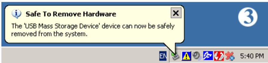
3. Disconnect the USB converter cable.
