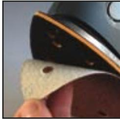
**Caution.** Take care to regularly clean out the build up of dust on the platen underneath the sandpaper and not to let the sandpaper wear completely down before replacing it. Failure to observe these two precautionary measures can lead to damage to the hooks and loops on the platen and the sandpaper will not attach properly. If the platen is damaged, it can be replaced at an authorised service centre.
