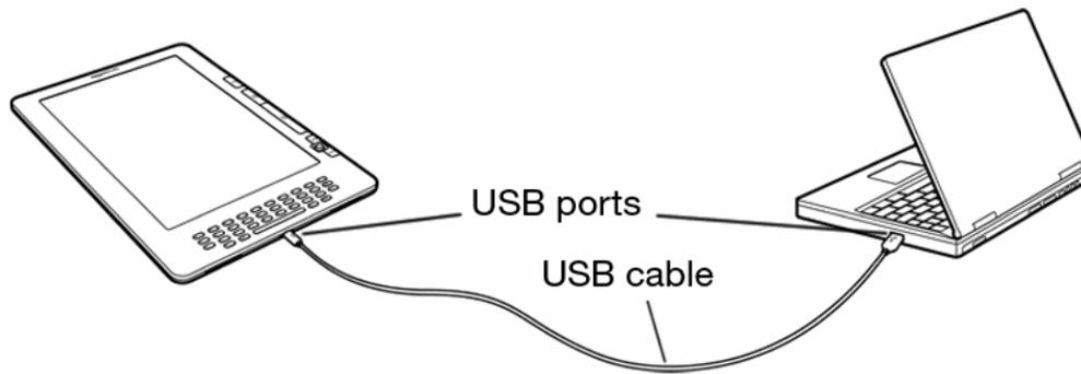
When you are connected to your PC, your Kindle will go into USB drive mode and its battery will be recharged by the computer. Your Whispersnet service is temporarily shut off and you will not receive any of your subscriptions while in this mode. Also, your Kindle is not usable as a reading device while you are in USB drive mode, but will return right to where you were when you un-mount the device from your computer.
