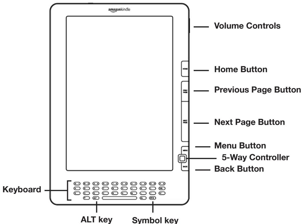
To select a particular item such as a menu option or a specific word in your reading material, move the 5-way controller up, down, left, or right to highlight your choice and then press to select.
